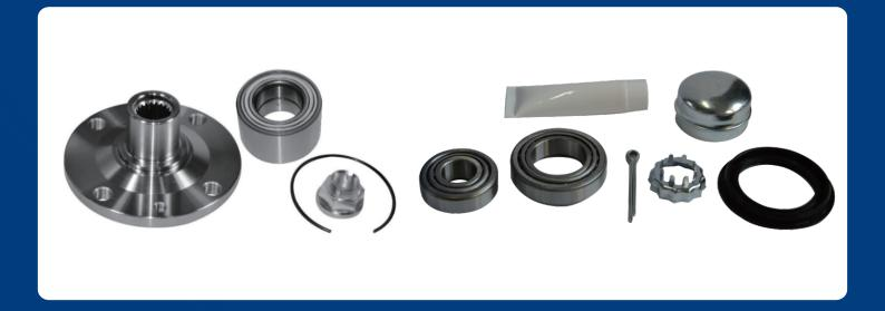
I Flanges get axial run-out due to thermal loads which leads to brake judder. As the workshop needs to disassemble the flange and bearing, repair kits allow to renew the flange during wheel bearing repair without extra work.
